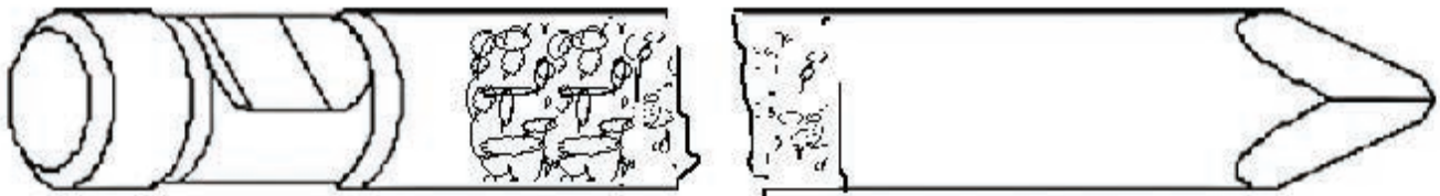
Fig. M-12 Tool Bit Failure
