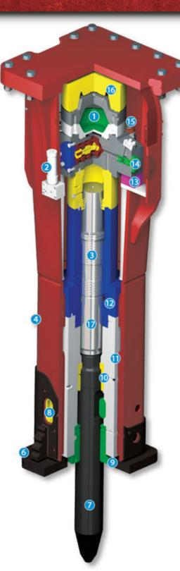
9 Field Replaceable Tool Bushings Slip-fit bushing allows owner to change bushings without the need of special tools. The Power Cell does not need to be removed from the housing to replace the bushing. 10 All-in-One Upper Bushing and Thrust Ring Integration
